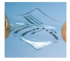
A fabrication method is introduced that utilizes masked deposition and selective wetting to produce hyperelastic electronic circuits that are composed of a thin elastomer film embedded with microchannels of liquid-phase gallium-indium (Ga-In) alloy. This method enables geometries that cannot be produced by injection and allows for the automated, high-volume production of Ga-In-based stretchable conductors.
